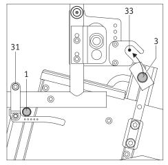
• Once the lower bolt [1] of the viamobil is fully seated in the lower holder [31], slightly lift up the viamobil.
